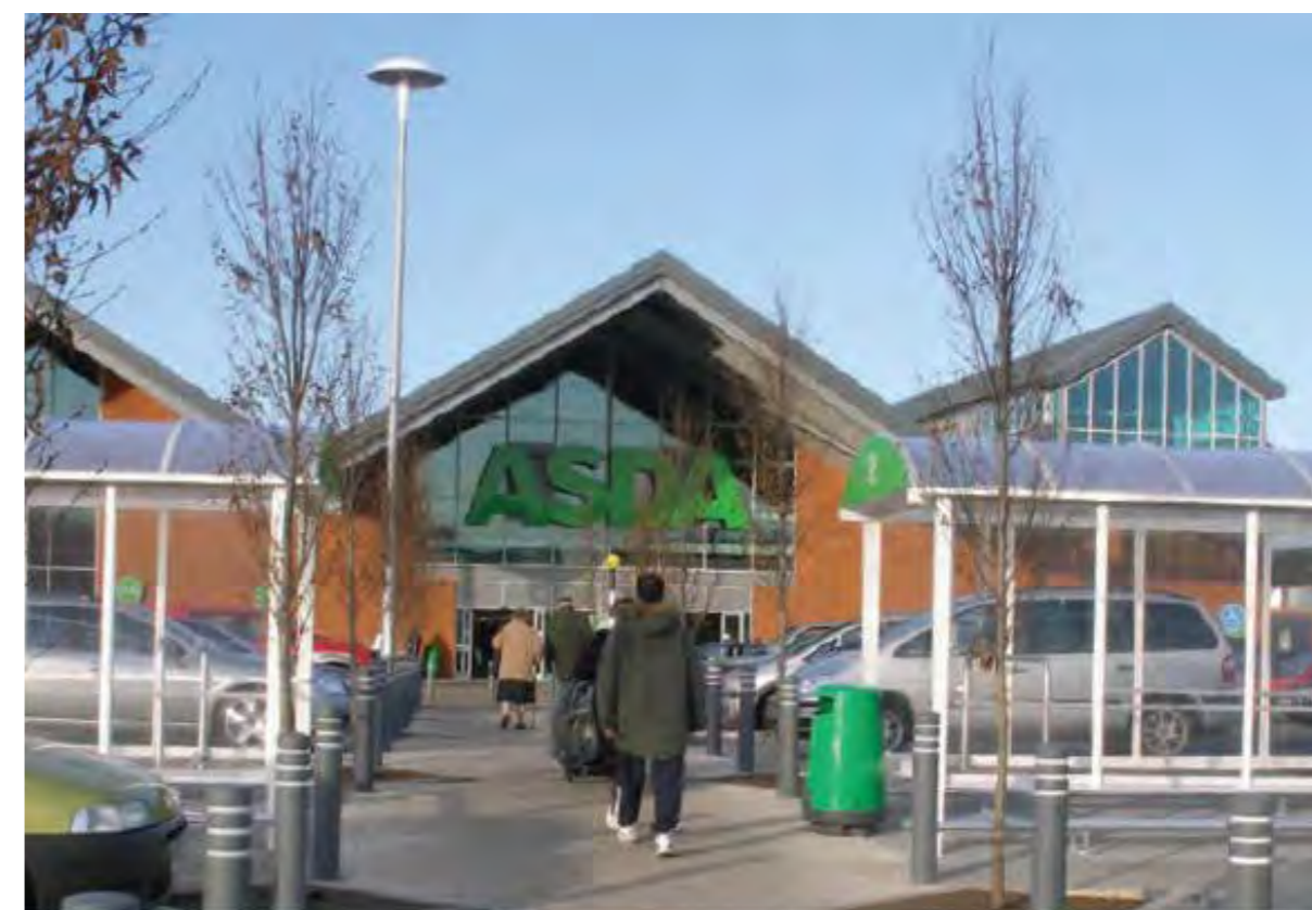
Figure 168: Large span foodstore with structural bays expressed and south facing walls recessed to create shading. Note also large, glazed areas allowing daylighting and creating an active frontage.
